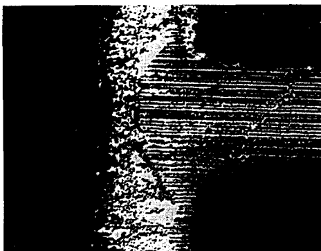
Fig. 3. Grid node of a concast Pb-1.8Sb grid (shoe side) showing extended surface porosity due to insufficient molten lead filling of the casting-drum grooves.
