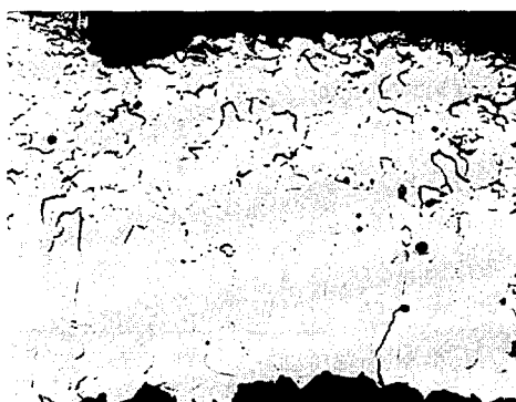
Fig. 6. Grain structure ( \times 100 ) of a concast Pb–0.06Sr–0.25Sn alloy. The cross section exhibits columnar grains on the drum side (bottom) and finer more regular grains on the shoe side (top).
